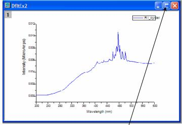
Above is an uncalibrated FluoroMax<sup>®</sup> lamp-s¢an. The main peak ought to be at 467 nm, but here appears near 480 nm.
