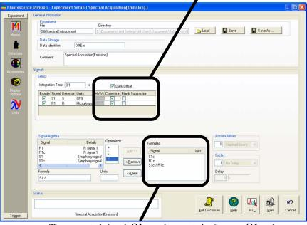
The corrected signal, S1c, and corrected reference, R1c, along with their ratio, S1c/R1c, all must be included in the Formulas list in the Signal Algebra area. If unchecked,  $S_{\text{dark}} = 0$ ,  $S_{\text{blank}} = 0$ , and Correction-factor file = 1
