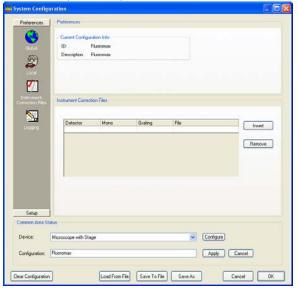
7 Choose the detector from its drop-down menu, the monochromator from its drop-down menu, and the grating from its drop-down menu:
