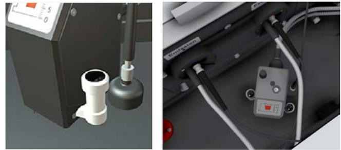
Fig 22: Schematic of the Quick-Fix holder (left) and actual image of the TRF-optic head in the instrument (right).
