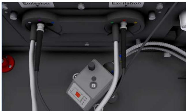
Figure 21: Turn the TRF optic head 45 degrees
