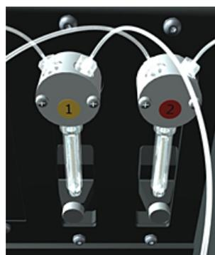
Figure 34: Reagent injectors
