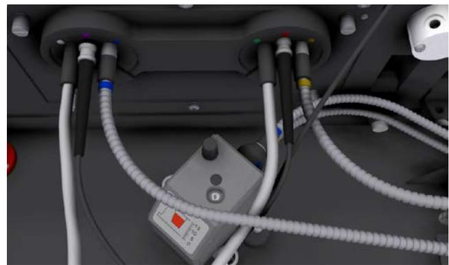
Fig. 23: Final look of the installed TRF optic head and light guides. Note: The excitation light guide must be positioned BELOW the black thin light guide of the absorbance spectrometer!
