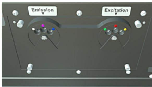
Figure 29: Filter change / filter installation: Loosen the 4 screws
